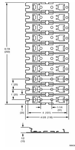
Figure 1. CRC9000 Mounting Strap (10) dimensions in inches (mm).
